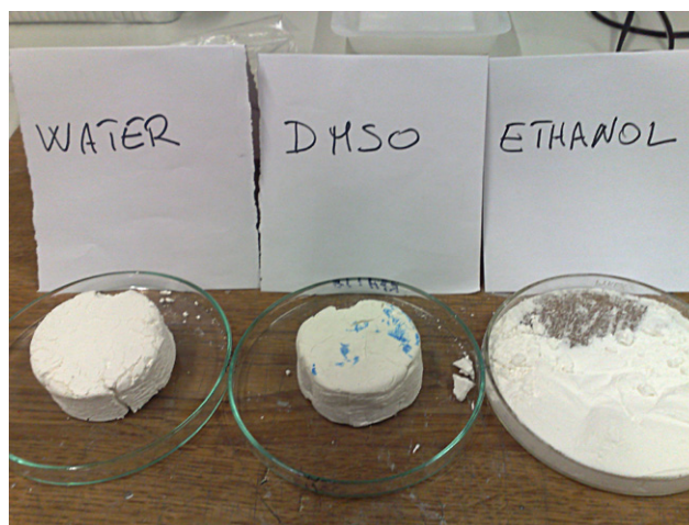
Fig. 3. Cylinders of water, DMSO and ethanol/MCC pastes after freeze-drying. The ethanol cylinder did not preserve the formed shape and crumbled back to powder during handling.
